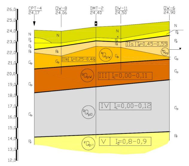
Figure 1: A standard geotechnical cross-section: OW – borehole test (reference method), CPT – cone penetration test, DMT – dilatometer test; (N – fill, Gp – sandy clay, Pd –fine sand, wn – moisture content, ID – relative density, IL –liquidity index)
